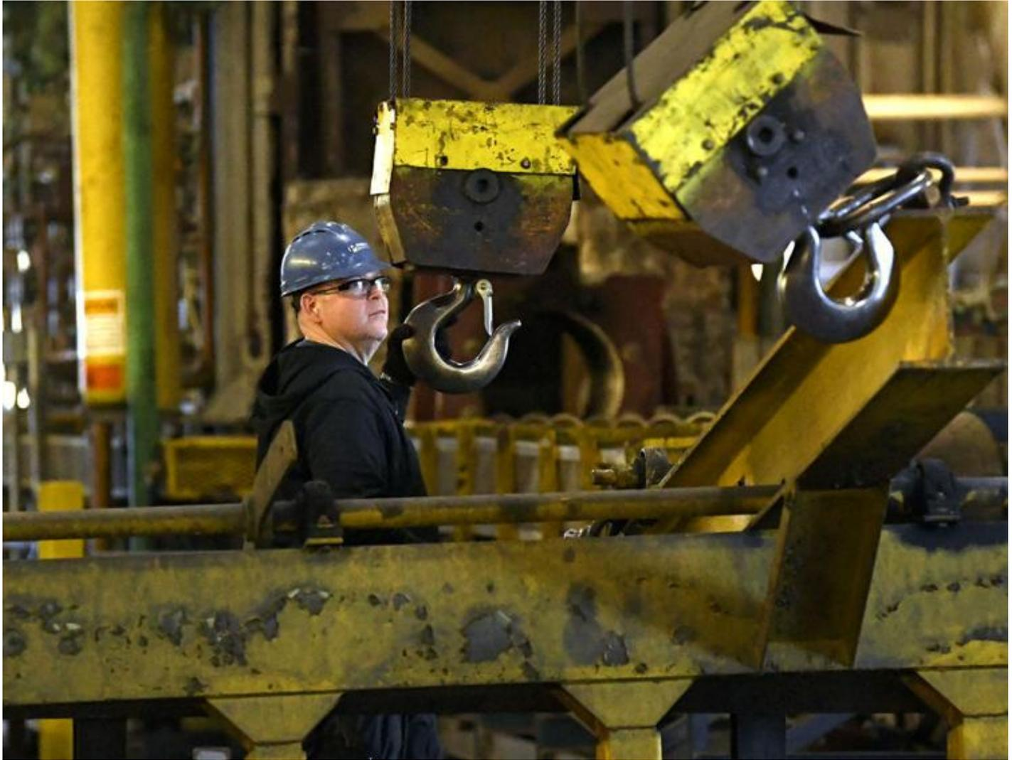
Keith Lamoreaux, a furnace operator with Primus Pipe & Tube in Wildwood, prepares equipment that will cool stainless steel tubes that have been heated to 1,950 degrees Fahrenheit.
